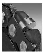
Do not judge the usability of the chain on visual appearance alone. It can have a few cutters with broken or missing carbide tips or many cutters with small chips of carbide missing and still cut very well... Or it may not have any broken or chipped cutters, but cuts slow because it has become dull. The only true determination should be based on how the chain cuts. If you are in doubt, make a test cut to determine the chain's performance.
